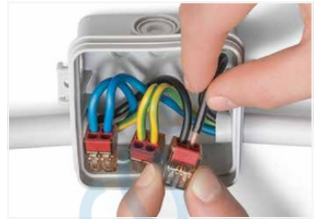
Termination: Insert stripped solid conductor until it hits backstop.
